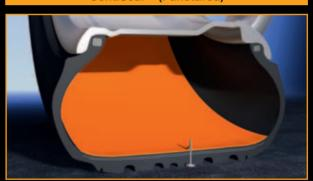
A ContiSeal™ tyre contains a sticky, viscous layer that covers the inside of the tyre tread. It provides an almost instantaneous seal around any penetrating object (up to 5 mm in diameter in the tread area), trapping the air inside, keeping the tyre inflated and your car mobile.
