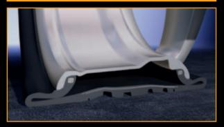
When a puncture occurs with a standard tyre the sidewall can become crushed between the rim and the road causing a potentially dangerous situation such as a blowout or the tyre slipping off the rim.
